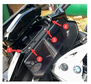
To remove the TFT screen simply open the phone compartment (after raising the screen to allow access). Remove the Torx 25 screws marked 2 and3 (left). Carefully grip the screen in the centre and tilt away from the phone compartment at the top. The screen should lift away and expose two connectors. The larger one requires thumb pressure on the catches to release and the smaller one simply pulls out.
