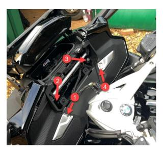
Once the TFT screen is removed as above, there will be two further fasteners for each side's speaker panels marked 1 - 2 (LH) and 3 - 4 (RH). (Shown Left).
